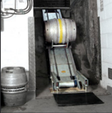
Sloping CellarLift with 22 gallon keg
