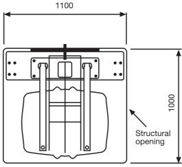
Recommended for a minimum clear vertical shaft 1100mm x 1000mm
