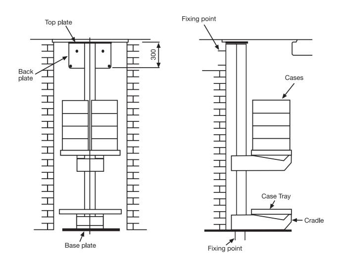
This hatch houses the hoist mechanism and requires 1500mm clearance above it
