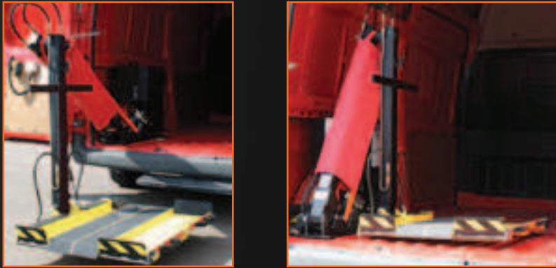
Automatic flaps ensure the load remains secure on the platform
