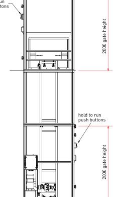
1480 structural opening\* IAI DEL 1300 usable platform 2000 structural opening\* 260 \*Minimum structural opening Drawing dimensions in millimetres
